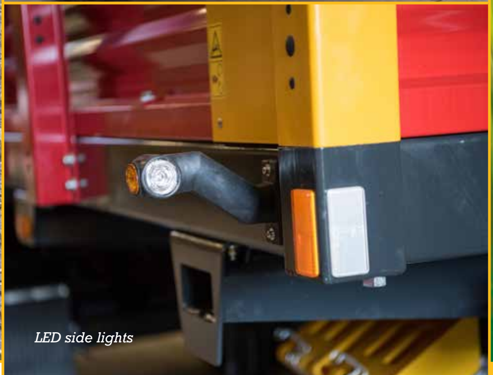
Bumper with LED roadlights and mudguards
