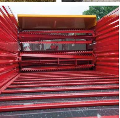
The Feedo's are fitted with two or more open and aggressive silage beaters. The beaters have different diameters and run at different speeds as standard. In this way an outstanding distribution and mixing of the different sorts of silage and feed are guaranteed. The beaters are mechanically driven from the power takeoff (PTO). Due to the special Feedo forage box-feeder beaters the feed is distributed evenly and without structure loss, whereupon it will be discharged by the cross-conveyor.
